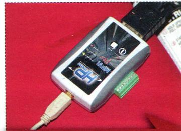
The HP Tuners programming interface is a durable and cost-effective tool for Home Tuners to use, and like all of its kind has built in 'black box' logging to gather hours of data during normal driving without you even knowing it's there
