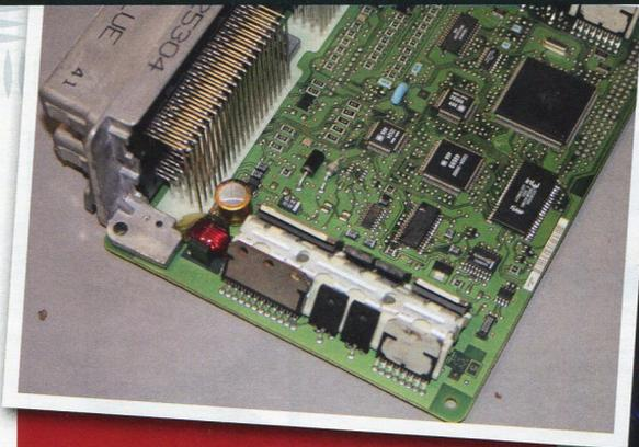
LS1 engine management is capable of having custom written operating systems loaded into it that are far superior to the factory MAFless offerings, even those used in the GTS
