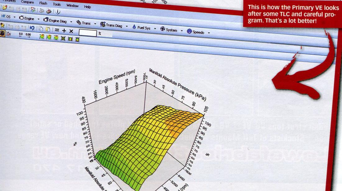
required to get the values right. The first thing we do is to remove the 'Himalayas' which is my fond term for the massive peaks and troughs that exist in the factory Primary VE table. These aren't specifically dyno selected number designed to make the car run best, but rather are overlooked and ill-regarded values that don't do an awful lot. If you have any doubt then move your eyes over to the supplied graphs and have a look at the peaks and troughs in the stock version!
