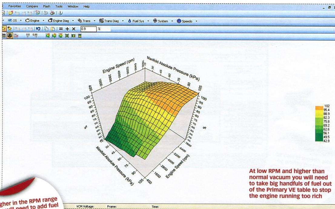
At low RPM and higher than normal vacuum you will need to take big handfuls of fuel out of the Primary VE table to stop the engine running too rich
