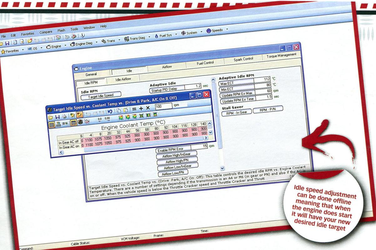
**Idle speed adjustment can be done offline meaning that when the engine does start it will have your new desired idle target**
