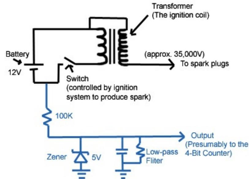
An introduction to Volts, Amps, and Ohms can be found [here](#). The transformer in the diagram is the ignition coil (concise documentation on what transformers are and how they work can be found [here](#)). Its purpose in the ignition system is to create high voltage current. The high voltage is necessary for the current to "jump across" the contacts of the spark plug, producing the spark responsible for fuel combustion.
