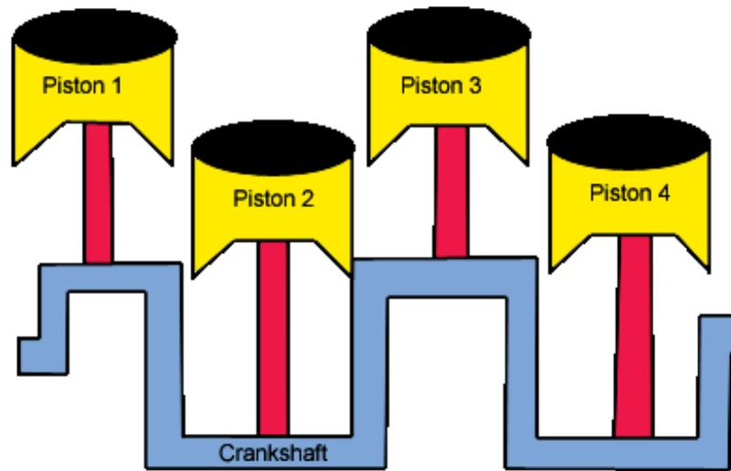
If Piston 1 has just completed its compression stroke, Piston 3 has just completed its exhaust stroke. If Piston 2 has just completed its combustion stroke, Piston 4 has just completed its intake stroke. In addition, the combustion stroke of one cylinder results in a 180 degree revolution of the crankshaft. Because of this, it takes combustion in two cylinders for one complete revolution of the crankshaft.
