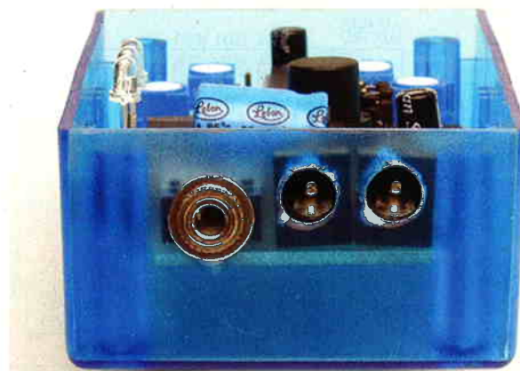
From the left, thermistor 3.5mm jack socket and the DC sockets for output to charger base and plugpack input.
