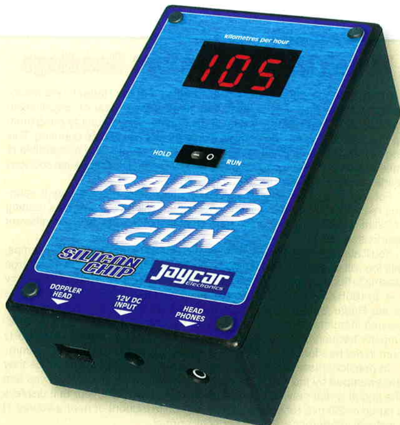
The counter/display unit fits inside a standard plastic case. This case will be supplied pre-drilled and with a screened panel as part of the Jaycar kit.
