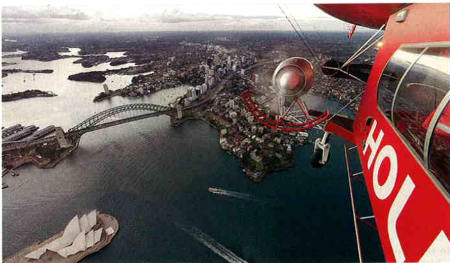
This photo, in flight over Sydney Harbour, shows one of the two 180 BHP Lycoming motors attached to the rear of the gondola. They chew through 91 litres of Avgas each hour! (Photo by Peter Murphy).
