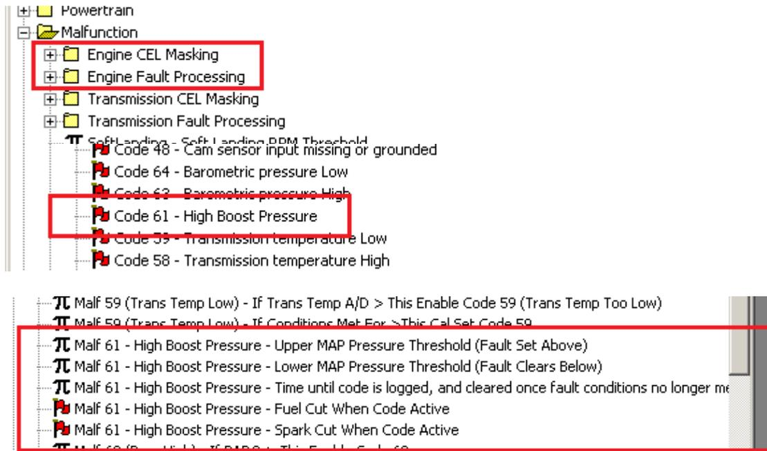
A fault will be set if MAP pressure exceeds the upper threshold for the time threshold. The fault will be cleared when the MAP pressure is below the lower threshold for the time specified. The fault will be stored in the malfunction history.
