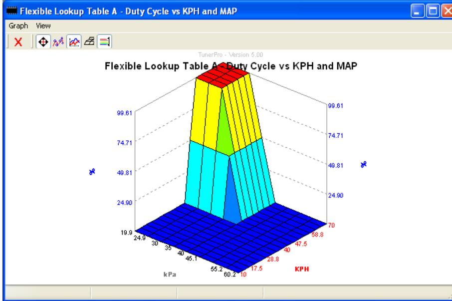
Another use for the above solenoid would be to use as a boost solenoid and the axis could be rpm's v's MAP to allow control over boost levels etc.
