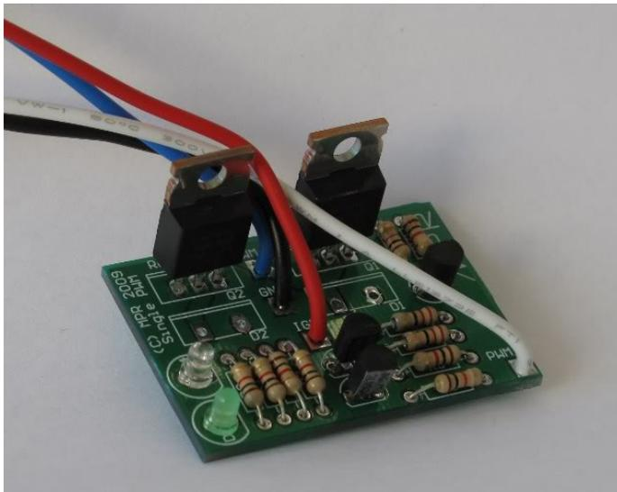
This device is a voltage controller which works in conjunction with the flex tables output to speed up/slow down a 12v motor.
