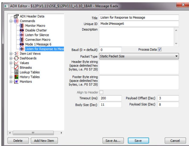
The main items that need changing are body size and payload size, and these change dependant of how many items you have selected above. For the above message 6 configuration we have 13 bytes of data to collect so we need to increase the payload size to 13 and increase the body size to 16.
