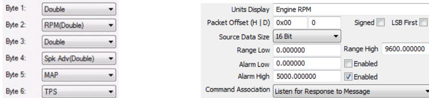
So as you can see in the first 6 bytes of the message 6 settings we have byte 1 & 2 and byte 3 & 4 are both doubles and the byte 5 and byte 6 are both singles. So we set the adx to use 16 bit for 0x00 offset (engine rpm) and 16 bit for 0x02 offset (spark advance) and then 8bit for 0x04 offset (map) and so on.
