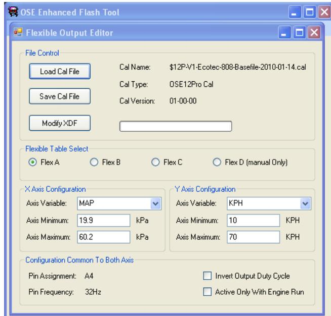
Once the axis are setup there are some other options down the bottom that can be adjusted, inverting output means whether 100% duty cycle is on or off, and active only with engine running is fairly self explanatory.
