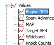
So the default settings of this adx are a good starting point, but we need to make sure they have the right offsets and to do this click on each, so Engine RPM is offset 0x00 and 16 bit, so this is fine.
