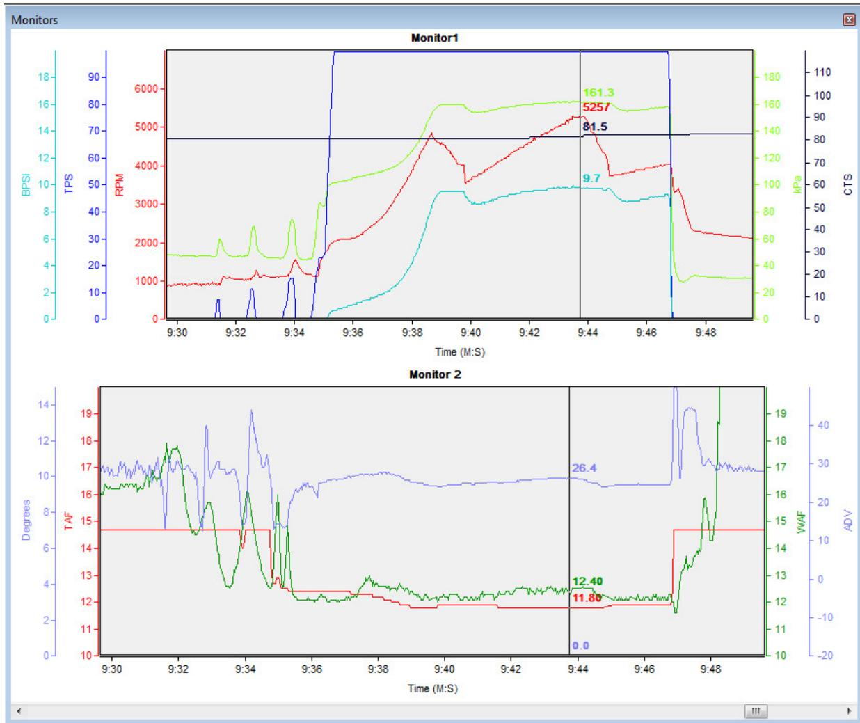
Just for reference in the top window the aqua line (BPSI) is boost PSI and is a calculation of map kpa converted into PSI and is used to ensure waste gate is set right.
