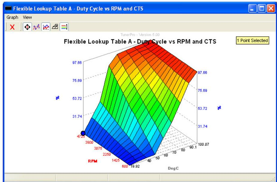
Likewise if the engine is stone cold and revved to 6000rpm it will use the low temperature values of the left hand side of the graph.
