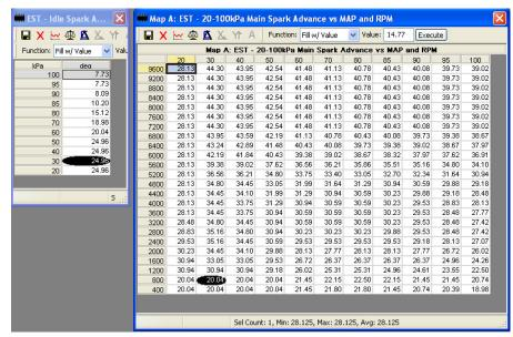
engine is switching between tables it will be changing the timing, this can often be seen as an engine at idle with the spark timing gauge jumping all over the place.
