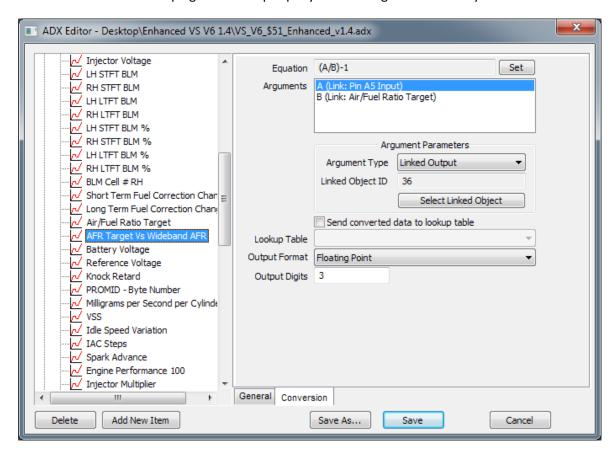
This will then just calculate the change needed to be made for the injector multiplier table to correct the fuelling compared to what is commanded, for EG 14.7 Commanded, 15.84 via Wideband so 7.76% Richer is needed.
