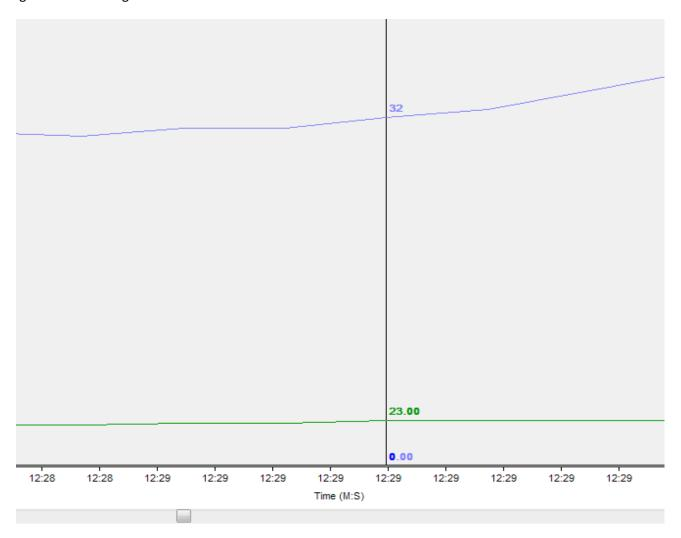
Third Example you can see KAL triggering Twice but we receive no knock or knock retard indication and timing has been removed, this is due to the fact timing retard and knock bitmask is only offered on the data bus for a small amount of time and we may miss picking up the packet, this is the big advantage of KAL you can clearly see that knock was present.
