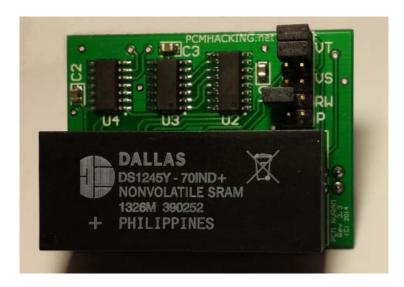
This is a typical PCMHACKING.net PCM NVRAM board. It is similar to the ECM NVRAM, but there are differences. The late model cars do not have any settings for number of cylinders on the memcal, so you will not find those settings here. There is also no knock filter required, so there is no need to connect an original memcal.
